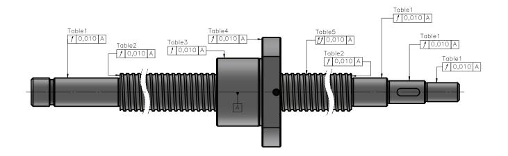
Table 2: Radial run-out bearing seat related to the centerline of screw groove and radial run-out of journal diameter related to the bearing seat.
